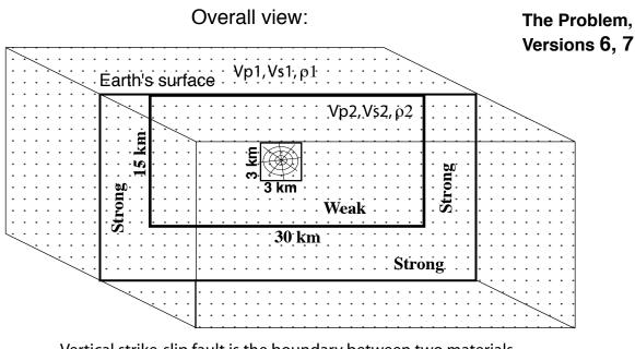
Vertical strike-slip fault is the boundary between two materials. On the far side of the fault, Vp, Vs, density = Vp1,Vs1, $\rho$ 1 On the near side of the fault, Vp, Vs, density = Vp2, Vs2,  $\rho$ 2
