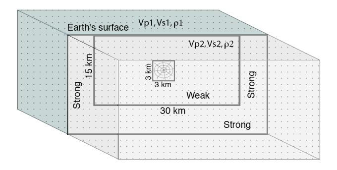
Vertical strike-slip fault is the boundary between two materials. On the far side of the fault, Vp, Vs, density = Vp1,Vs1, $\rho$ 1 On the near side of the fault, Vp, Vs, density = Vp2,Vs2, $\rho$ 2
