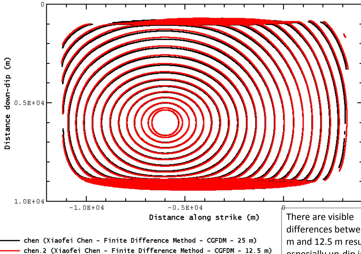
There are visible differences between 25 m and 12.5 m results, especially up-dip in the mode III direction. This is maybe due to the low velocity.
