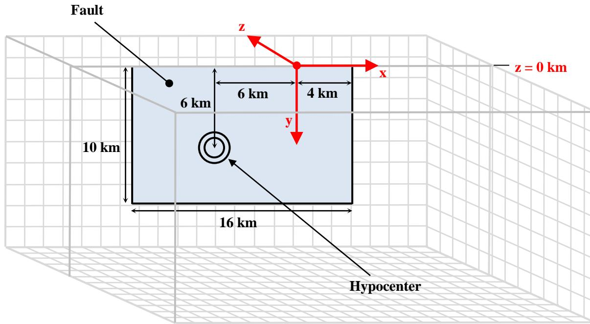
Right-lateral strike-slip fault in an elastic half-space, with a low-velocity fault zone.
