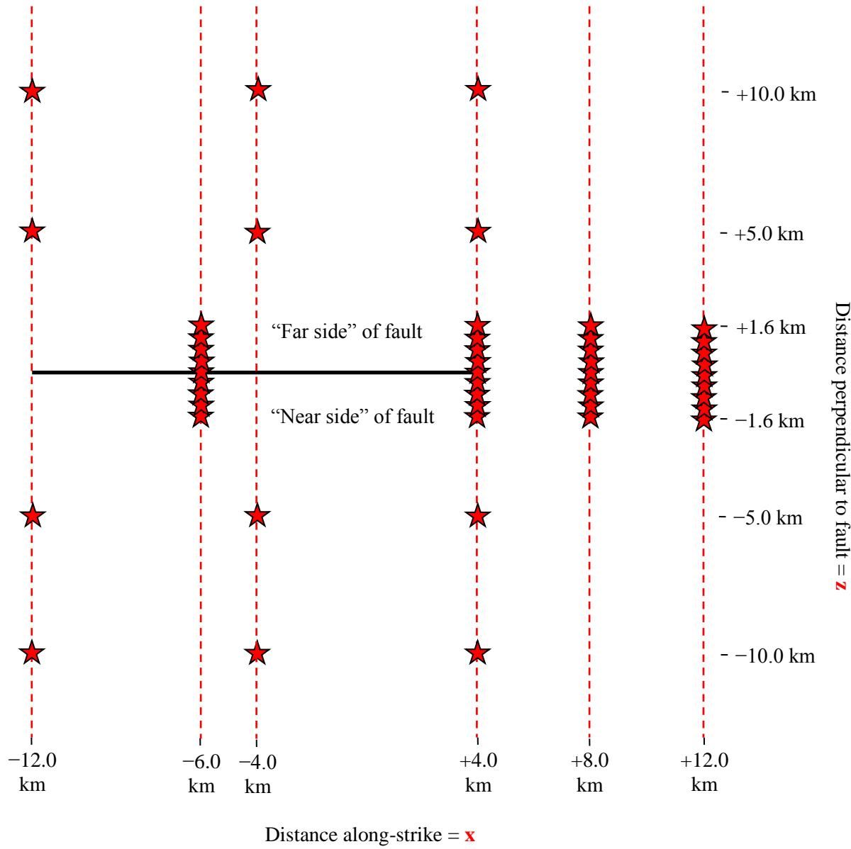
Modelers are asked to submit displacement and velocity as a function of time, for 48 stations on the earth's surface.
