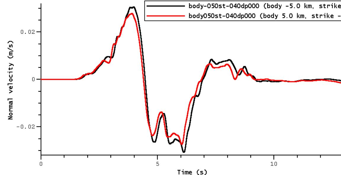
If the material properties were symmetrical, the normal velocity would be the same at each mirror-pair of stations.
