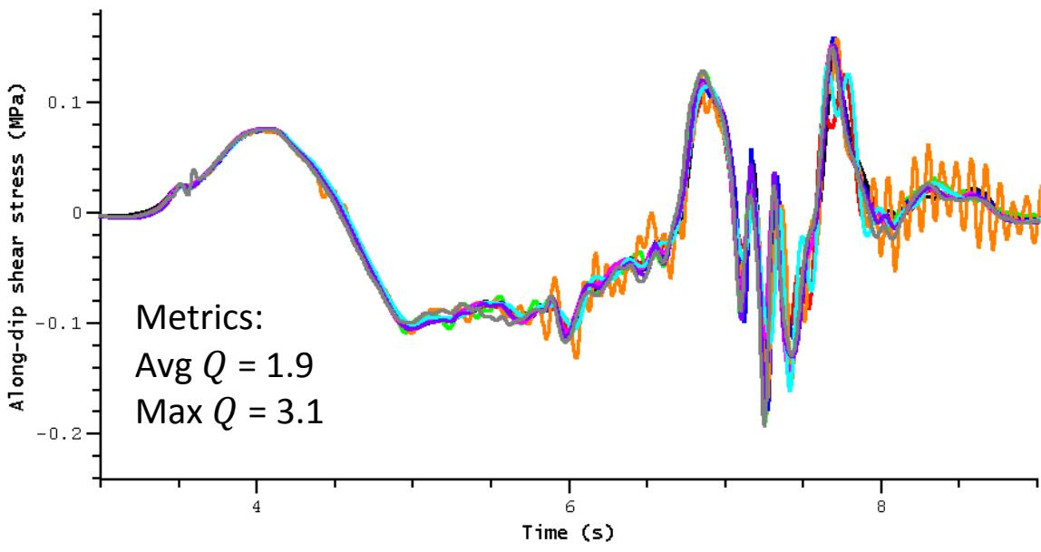
Vertical shear stress agrees very well despite being small and having a complicated waveform.
