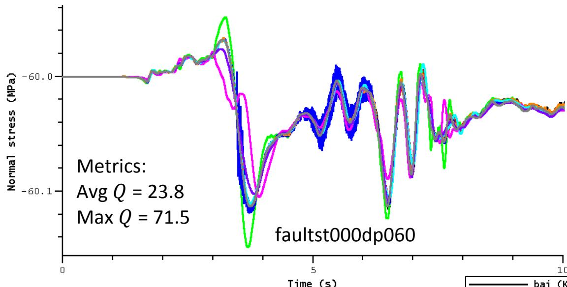
Normal stress can only vary because of the slightly different material properties on the two sides of the LV zone. So the effect is small: about 0.3% and 0.07% at the two stations shown.
