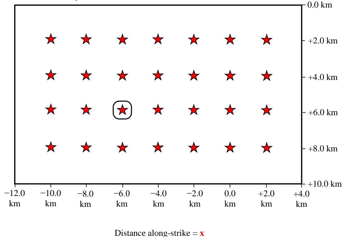
Modelers are asked to submit slip, slip rate, and stress as a function of time, for 28 stations on the fault.
