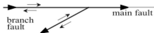
(b) Turn of rupture path through obtuse \phi angle while continuing on main fault (never favored by stress field)
