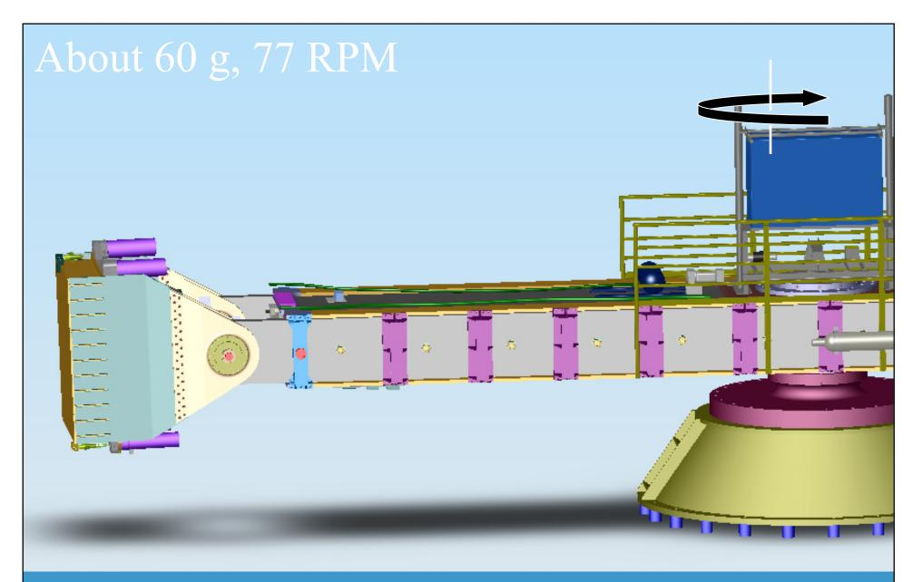
The centrifugal acceleration increases the vertical stress profile in the model such that the vertical stress in a 0.5m thick soil layer approximates a 30m thick prototype profile.
